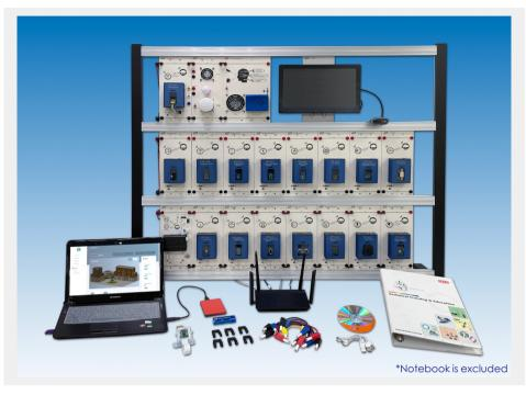
IOT-110 is a platform that integrates the training of edge computing, AI., and IoT. Its system consists of sensor modules, edge computing modules, and AI computing accelerators. The course provided is structured coherently and clearly, and the concepts of sensors, networks, and applications can be introduced progressively and thoroughly. With this system, users shall be able to deploy various smart applications of IOT and edge computing.
